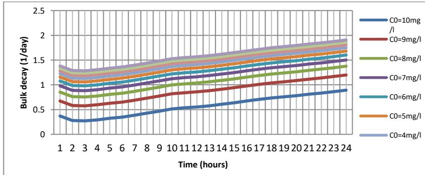
**Fig 4** bulk decay for different assumed initial concentration.
