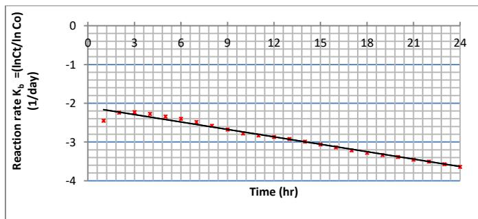
**Fig 5** reaction rate of bulk decay " $k_b$ " for study water network found in Lab.
